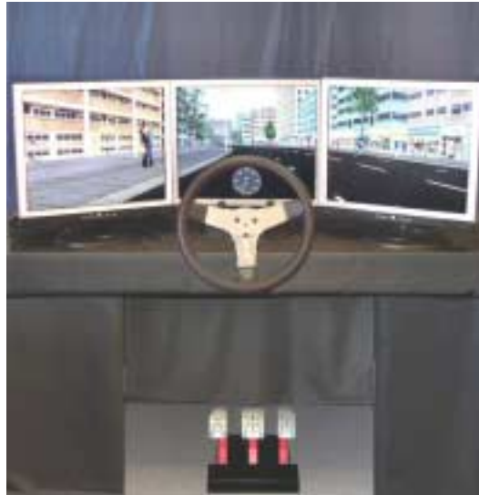
XP-300 with 3 channels and improved controls
